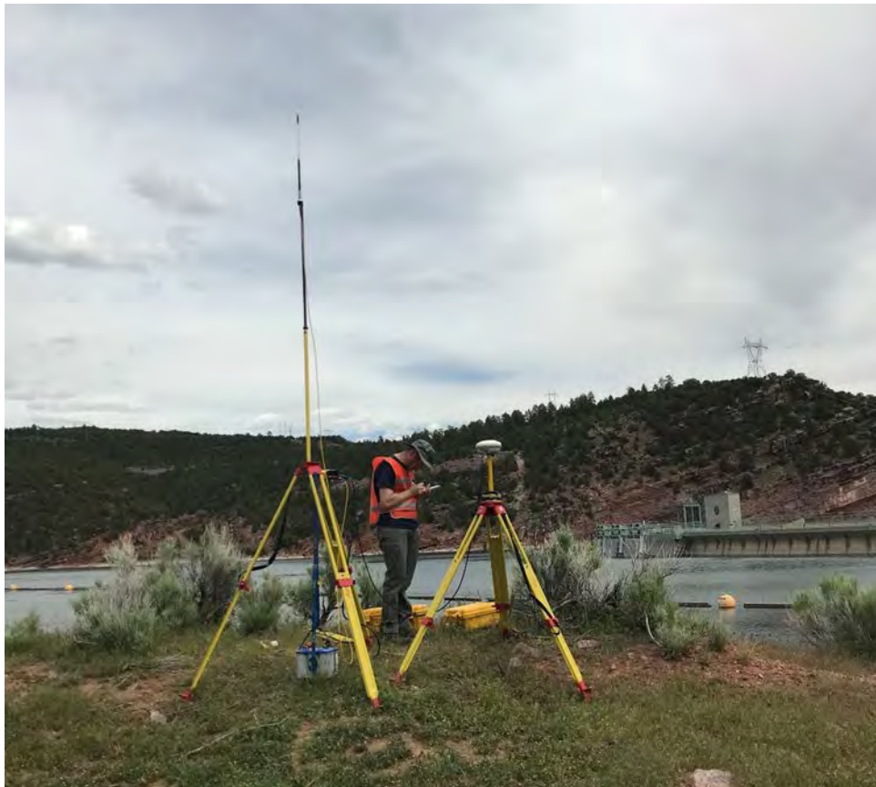
Figure A-2. The RTK-GPS base station set-up used during the survey Flaming Gorge Reservoir in Utah and Wyoming is typical of the set up used for other reservoir surveys.
