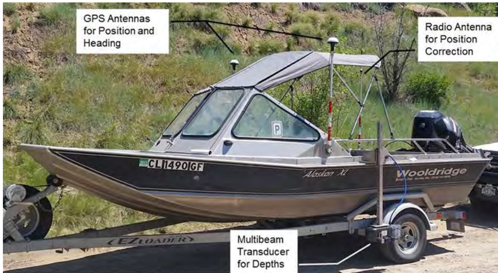
A-1. Wooldridge boat with RTK-GPS and multibeam depth sounder system.
